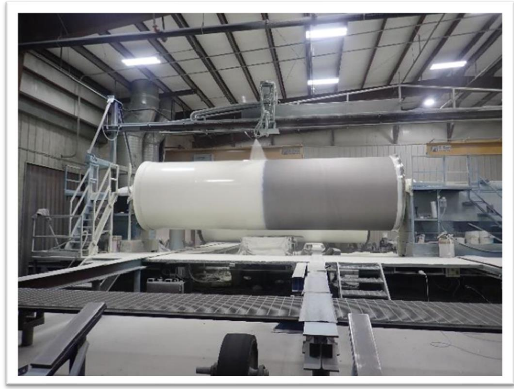
Polyurethane Coating Application
