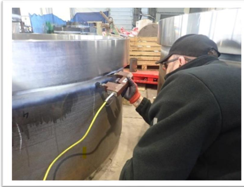
Magnetic Particle Testing (MT)
