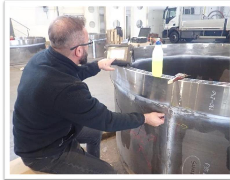
Ultrasonic Testing (UT)
