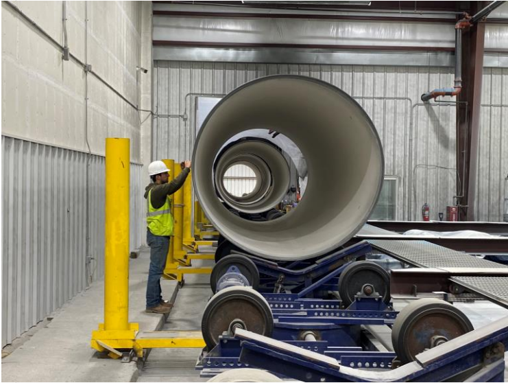
Pipe Quality Assurance – Coating Inspection Accurate
