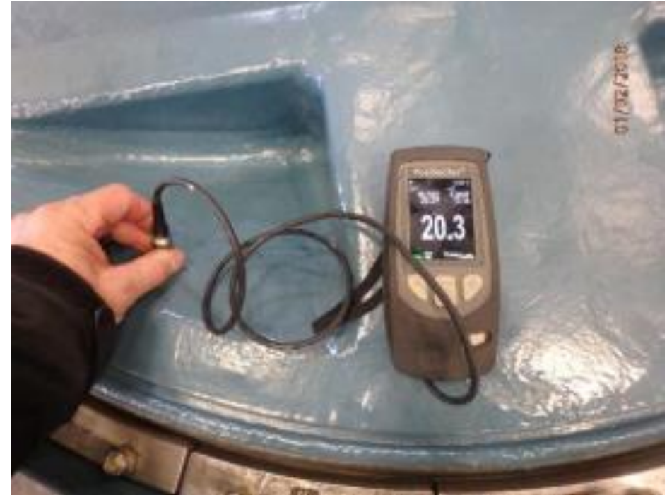
Coatings Quality Assurance Thickness Verification
