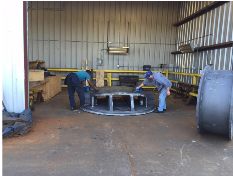
Non-Destructive Testing – Ultra Sonic Inspection of Casting Accurate
