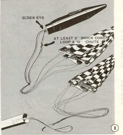
In preparing the Cineroc for flight, the parachute attachment point should be given careful consideration. The extreme versatility of the Cineroc becomes apparent when a little thought is given to the many attachment variations possible. The rear adapter attachment method illustrated at the left is standard and is recommended for the first few flights. An 18' parachute and shock cord is supplied with your camera and should be assembled as shown.
