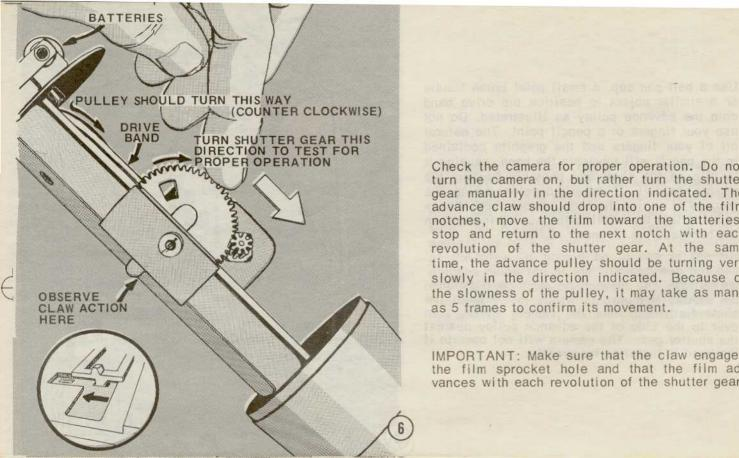
Check the camera for proper operation. Do not turn the camera on, but rather turn the shutter gear manually in the direction indicated. The advance claw should drop into one of the film notches, move the film toward the batteries, stop and return to the next notch with each revolution of the shutter gear. At the same time, the advance pulley should be turning very slowly in the direction indicated. Because of the slowness of the pulley, it may take as many as 5 frames to confirm its movement.
