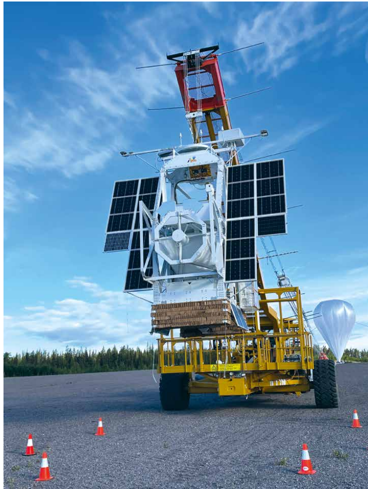
The Sunrise III observatory shortly before launch on the Hercules crane vehicle. The huge balloon in the background to the right is already partially filled with helium. During flight, it carries a load of almost three metric tons.
