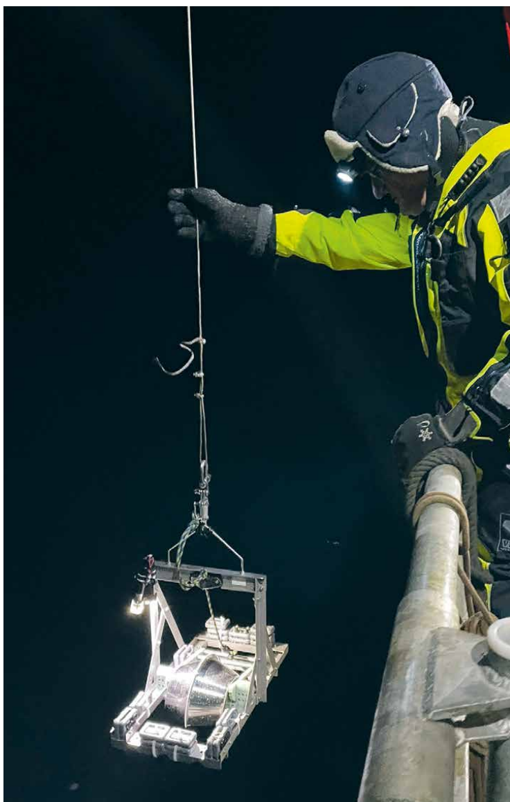
During the polar night in Isfjorden, Dirk de Beer uses a small crane to lower the Ellrott grab into the water. The device is a sediment sampler designed by the researchers. It is equipped with a flashlight and a camera to illuminate and view the seabed and the surrounding area, and to ensure that the device touches down on the sediment gently. Weights stabilize the device during sampling.
