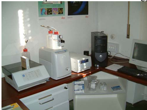
Fig.: the Ion Chromatography System (Dionex ICS90) at the GeoBio-Center LMU (for details see: www.geobio-center.de )
