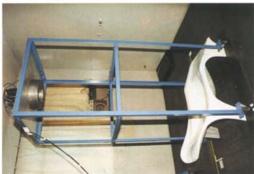
32. The improvised whole body counter used in Goiânia.
