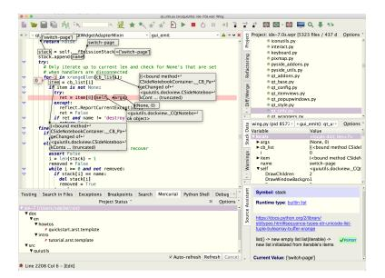
Wing Pro is a Python IDE that can be used to develop, test, and debug Python code written for the Django web development framework. The debugger works with Django's auto-reload feature and can step through and debug Python code and Django templates. Wing Pro also automates some aspects of the creation and management of Django projects and applications.
