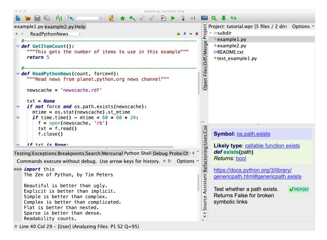
Tool and editor tabs can be dragged to rearrange the user interface, optionally creating a new split or moving them to a separate window. Right click on the tabs for a menu of additional options, such as adding or removing splits or to move the toolbox from right to left. The number of splits shown by default in toolboxes will vary according to the size of your display.
