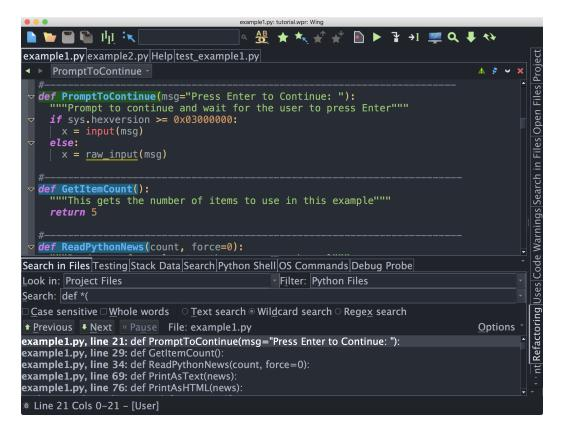
Before worrying about the details, try a simple batch search on the **example1.py** file. Select **Current File** from the **Look in** selector on the **Search in Files** tool. Then enter **PrintAs** into the search area.
