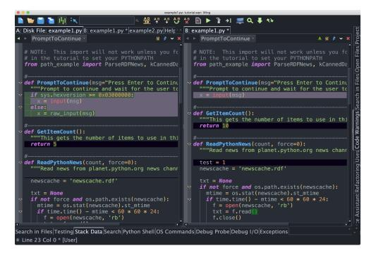
Use the **Previous Difference** and **Next Difference** items to move through the differences and the **Merge A->B** tool to undo unsaved changes.
