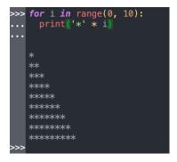
Notice that the shell removes common leading white space when blocks of code are copied into it. This is useful when trying out code from source files.
