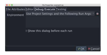
The most common use of **File Properties** is simply to set the command line arguments to use with the file. Try this now by bringing up **File Properties** for **example1.py** and set the run arguments in the **Debug/Execute** tab to **test args**.
