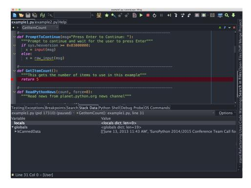
Notice that the debug status indicator in the lower left of Wing's main window changes color depending on the state of the debug process. Hover the mouse over the indicator to see detailed status in a tooltip.
