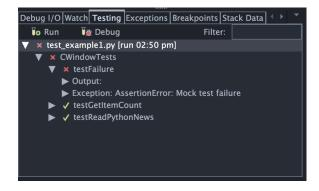
You can expand the tree to see details of the failed tests, including any output printed by the test and the exception that occurred. Double-clicking on the test results and exception will take you to the relevant code.
