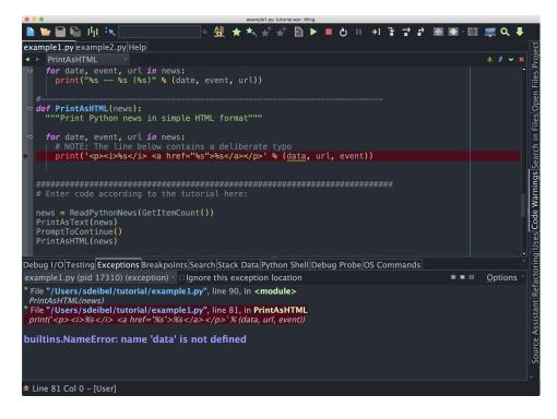
The **Exceptions** tool highlights the current stack frame as you move up and down the stack. You can click on frames to navigate the exception backtrace, showing the source code for each frame.
