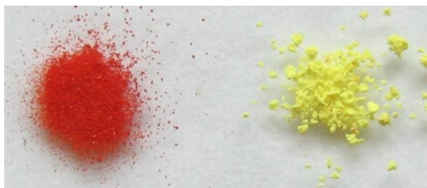
Figure 4 | Polymorphs of lead(II) oxide , litharge ( \alpha -PbO, left) and massicot ( \beta -PbO, right). Hubertus Giefers, public domain
