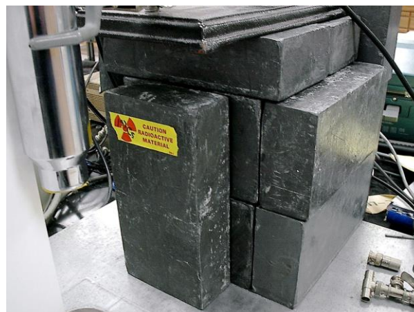
Figure 16 | Bricks of lead (alloyed with 4% antimony) are used as radiation shielding. [196] Loren Chang, public domain
