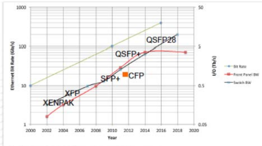
Figure 1: Ethernet data rate and switch bandwidth saturation: front panel bandwidth is saturating at about 5 Tb/s. (compliments of Nicholas Ilyadis, Broadcom)
