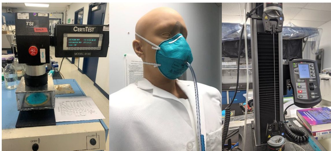
Fig. 22. Left: TSI 8130 Filter Tester for particle filter efficiency evaluation (see Table 2). Middle: Static advanced headform used for the manikin fit evaluation (see Table 3). Right: Instron 5943 Tensile Tester used for tensile testing of straps (see Table 4). Photo credits: NPPTL
