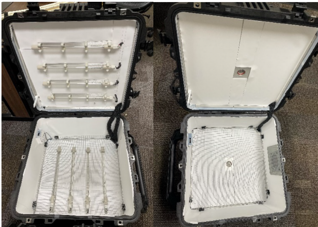
Fig. 7. The Hg lamp (left) and UV-C LED (right) chambers with reflective PTFE installed on the top, bottom, and side walls of each chamber.
