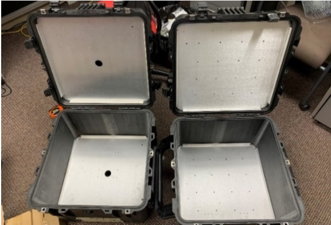
Fig. 5. The rugged box chassis with 46 \times 46 \times 46 cm interior dimensions and sheet metal dividers installed was designed for both LED and Hg lamp germicidal UV sources.
