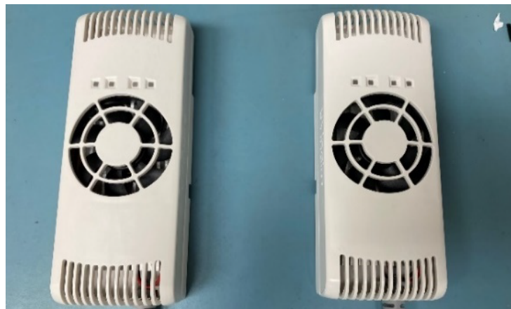
Fig. 3. UV-C LED housings with integrated heat sinks and fans irradiate targets from the top and bottom. Hot air is exchanged through vents in the chassis.
