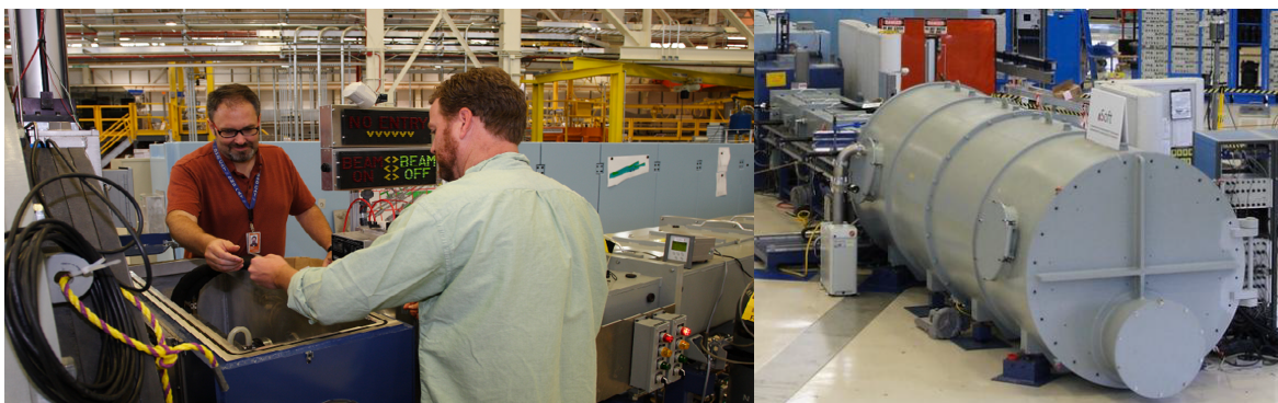
Fig. 9. Left: Researchers work collaboratively at the NIST Center for Neutron Research as part of the nSoft Consortium. Right: The 10 m small-angle neutron scattering instrument accessible to members of the consortium. The technique enables structural observations to be connected to processes used in manufacturing, including shear, high pressure, high temperature, and environmental exposure. It is foundational for the development of structure-property-performance relationships in solid materials, liquids, and mixtures [76, 79]. Credit: NIST.
