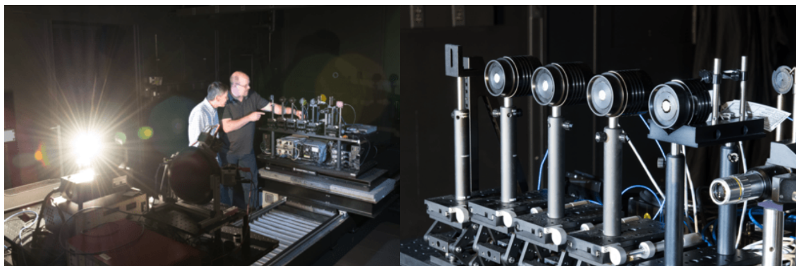
Fig. 8. Left: NIST's Yuqin Zong and Cameron Miller in the new, fully automated NIST photometry laboratory. Right: A row of identical photometers (light detectors) sitting on one of the new automated equipment tables in the NIST laboratory. Multiple identical detectors are used for each measurement so that researchers can ensure the readings are accurate [73]. Credit: Jennifer Lauren Lee/NIST.
