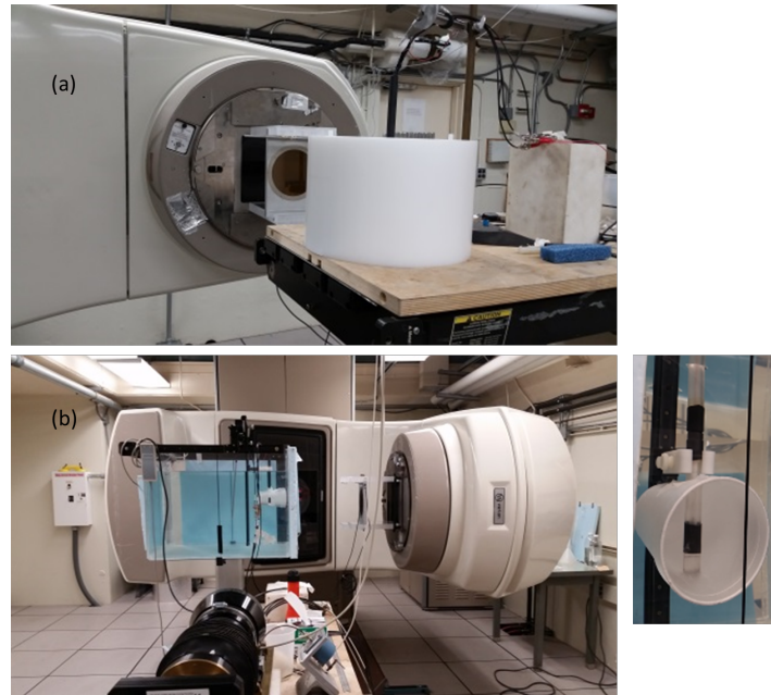
Fig. 3. Photographs of the measurement in the high-energy photon beam from a clinical therapy machine. The photon field size is 10 cm by 10 cm, incident horizontally. (a) Setup for the PE phantom, which has a channel along the central axis allowing insertion of the ionization chamber or the calorimeter core. (b) In-water phantom measurement, where the calorimeter is inserted vertically in the water, adjusting the distance to 10 cm water-equivalent thickness. The close-up photo, on the lower right, taken through the wall of the water tank, shows the submerged calorimeter core surrounded by a Styrofoam cup as a convection barrier.
