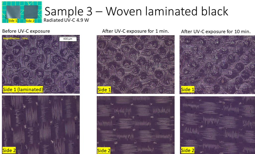
Fig. A.1.2. Endurance test #1 UV-C, sample 3: PPE coverall fabric (woven, laminated) showing no changes as examined using an Olympus BX53M upright light microscope.
