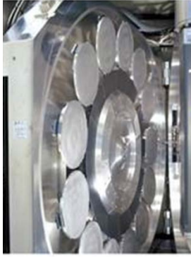
Fig. 1. The rotating disk and wafer holders in the batch type ion implanters (courtesy to SMIT).
