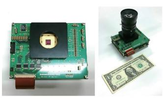
Fig. 1. Prototype CMOS sensor with quasi pixel-wise exposure.
