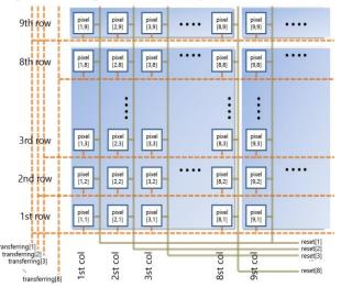
Fig. 2. Architecture diagram of CMOS image sensor with quasi pixel-wise exposure capability.
