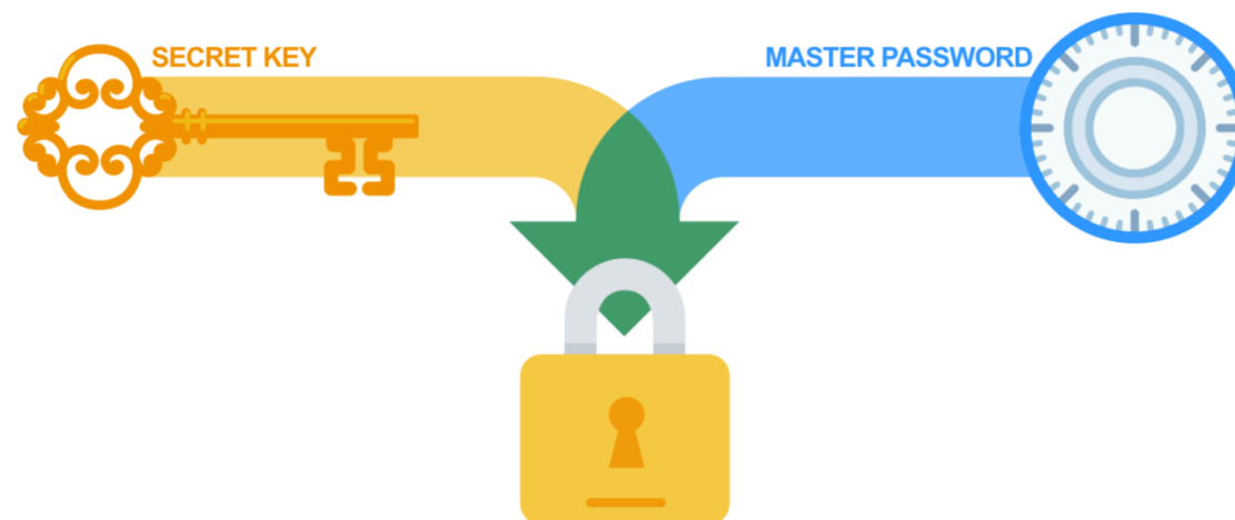
Figure 3.1: Two-secret key derivation combines multiple secrets when deriving authentication and encryption keys.
